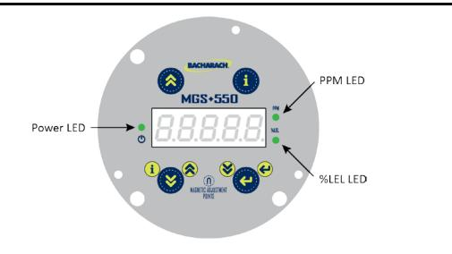
After the warm-up period, the instrument begins normal operation. The display toggles between the current gas concentration and target gas name.
