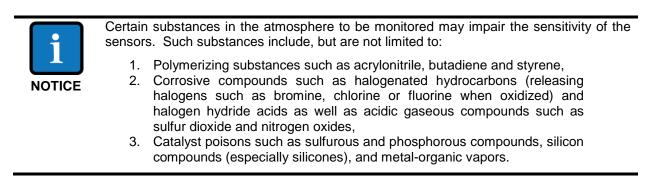
It may be necessary to check the calibration if the sensor has been exposed for a long time to a high concentration of flammable gases, vapors, or the above-mentioned contaminating substances.
