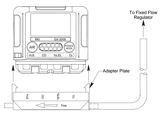
Figure 26: Installing the Adapter Plate, Auto Cal
