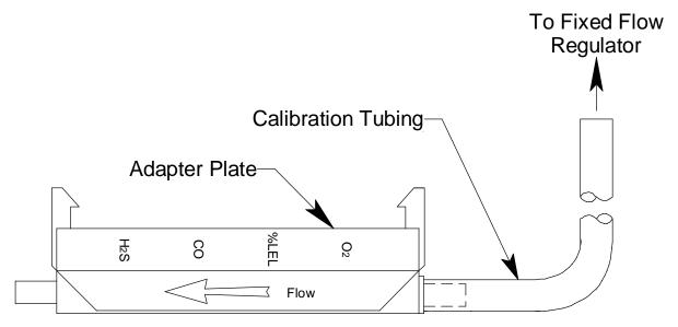
Figure 25: Calibration Kit Assembly
