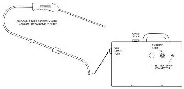
The gas-sample line can be up to **50 ft (15.2 m)** in length. All tubing bends should have a radius of no less than 5" to ensure proper airflow. If kinks or obstructions occur in the line the monitor may not function properly.
