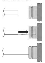
To connect the exhaust line to the exhaust port's PTC fitting, firmly push the appropriate tubing into the hole in the center of the connector until it seats in the connector. Refer to the figures at the left.
